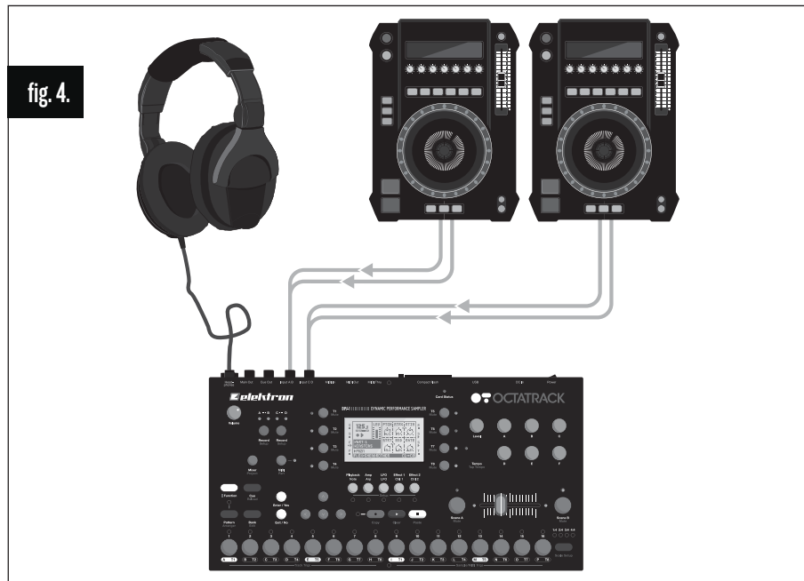
Fig 4. Two DJ decks are connected to the Octatrack inputs. The headphones output is set to monitor both the main and cue outputs. The crossfader is assigned to control the main output balance between the two incoming signals. The Octatrack can mix between the DJ decks by either using the DIR method or the Thru machines method.
